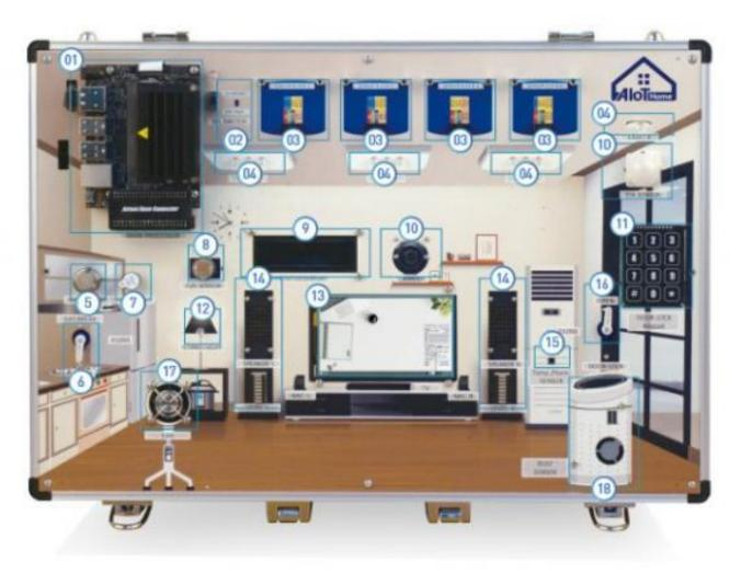
01 Main Processor 02 Connection Select Switch 03 Sensor Block 04 LED Block 05 GAS Sensor 06 GAS Break(Servo Motor) 07 Buzzer 08 CdS Sensor 09 Text LCD 10 Camera 11 Touch Keypad(3 x 4 key) 12 RGB LED 13 TFT LCD 14 Audio Block
